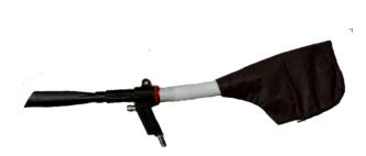
Wonder-Gun is a new type of air gun that uses compressed air for blow off, suction, and for transfer of materials. Wonder-Gun adopts the special jet system, which is a way of bringing out the full power of the compressed air. There are no worries that materials might get clogged inside the Wonder-Gun as it doesn't have any interior restrictions.
